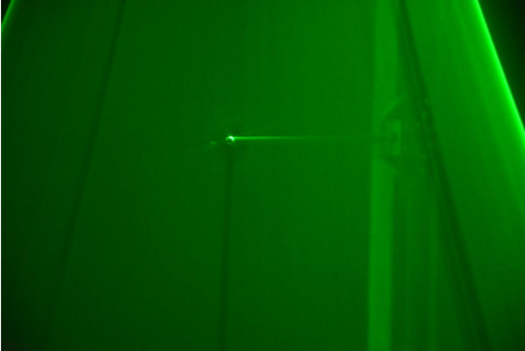
Figure 10 Image showing example of probe insertion during crossflow visualization at an angle of attack of 12 degrees and a tunnel set speed of 30 m/s at a location 14 chord lengths downstream of the vortex generator
